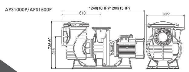
Self-Priming Pump: APS550P, APS750P Centrifugal Pump: APS1000P and ASP1500P
