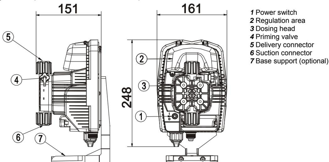
The parts in contact with the liquid have been chosen in order to guarantee perfect compatibility with most chemical products normally in use. Given the range of chemical products available on the market, we recommend checking the chemical compatibility of the dosed product and contact materials.
