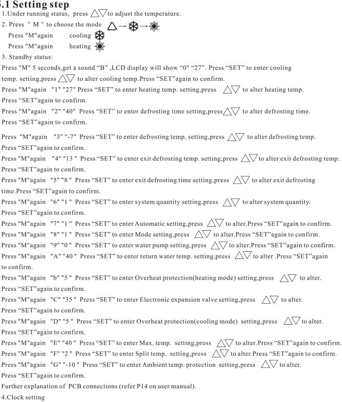
Under running or standby status, Press "SET" for 5 seconds, get a sound "B", press \times to alter hour, press "SET" again to alter minute. Press "SET" again to confirm.
