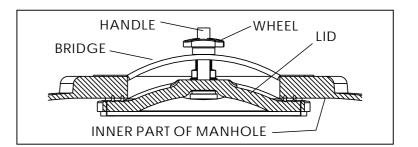
Introduce the lid in the manhole, leaving it leveled and centered. The lid must be supported by the handle, as this will avoid that it could fall into the tank and damage any of its parts.
