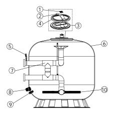
Notes:10\* E1050/E1200 should have 185mm x 8pcs and 233mm x 8pcs and 129mm x 8pcs of laterals 10° E1400 should have 185mm x 4pcs and 233mm x 12pcs and 129mm x 12pcs of laterals 10° E1600 should have 185mm x 8pcs and 233mm x 12pcs and 129mm x 12pcs of laterals 10° E2000 should have 185mm x 8pcs; 233mm x 32pcs; 129mm x 8pcs of Laterals 10° E2200 should have 185mm x 40pcs; 233mm x 16pcs; 129mm x 48pcs of Laterals
