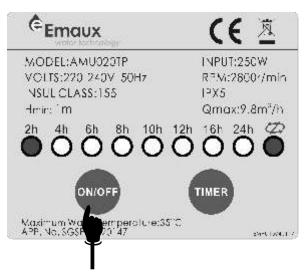
When the timer is set to 2h, the pump will operate and stop after 2 hours until the pump is switched on again.
