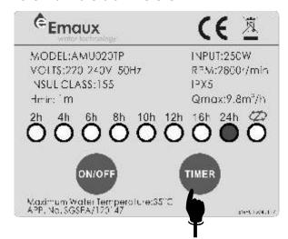
After turn on the pump, the default setting is 24 hours continuous operation. To set the desired operation period, this can be done by pressing the timer button (2h 4h 6h 8h 12h 16h 24h 2h).
