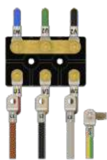
High Voltage WYE/STAR Connection
