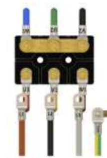
High Voltage WYE / STAR Connection
