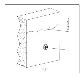
The flow rate required for the installation will determine the number of inlets needed. Three different diameters(14 mm, 20 mm and 25 mm) are available in the eye ball, so you can choose three different flow rates according the pool requirements:
