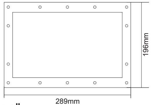
**Use the doubled side tape to fix the gasket to the pool wall.**
