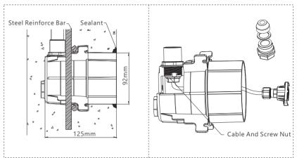
4. Insert the clamp ring into the niche before ceramic is applied. Wrap the power cord few round
