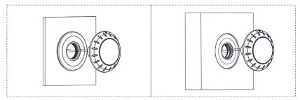
4. Screw light, Adjust the tightness by O-Ring, and "TOP" upwards.
