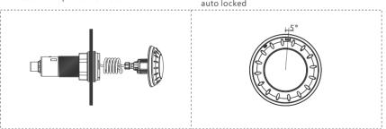
2. The niche and the concrete wall should be seal 3. Lead the power cord with connector through with sealant to prevent water get inside. the niche
