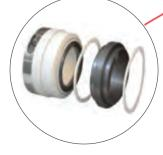
External type AISI-316L mechanical seal for highly corrosive fluids, static and rotating rings in SiC, spring and Polyester thermosetting powder coated power frame construction to prevent external corrosion
