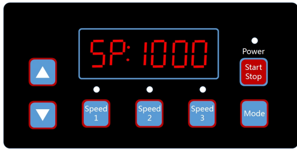
Speed Display ("SP:1000", indicate in speed RPM 1000)
